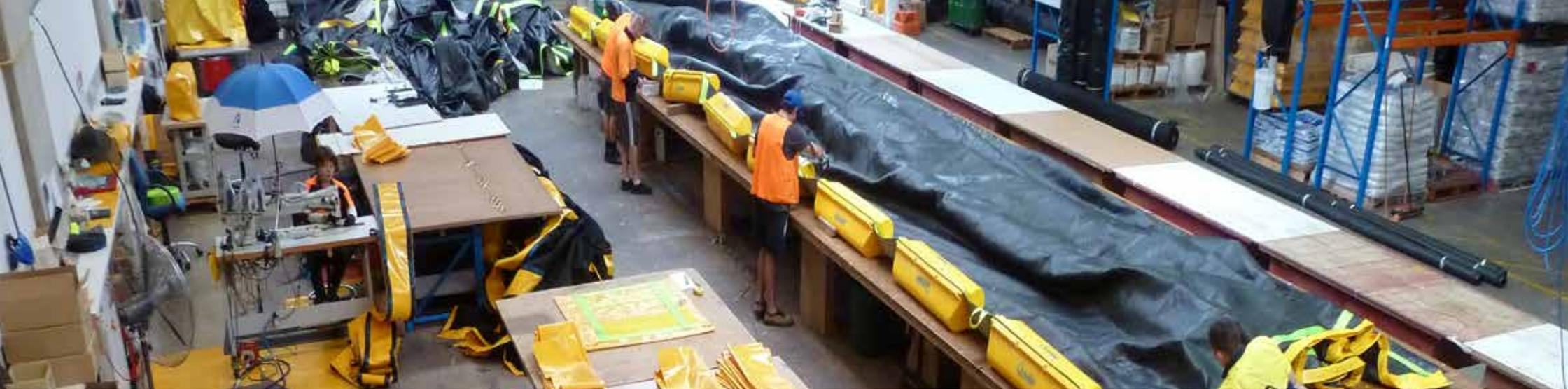
Floating curtains, baffles and various containment booms are examples of the most complex products we make. In producing these floating barriers we utilise a wide variety of materials and tools. The fact is, we produce over 30 other environmental compliance products using these common materials and components.
