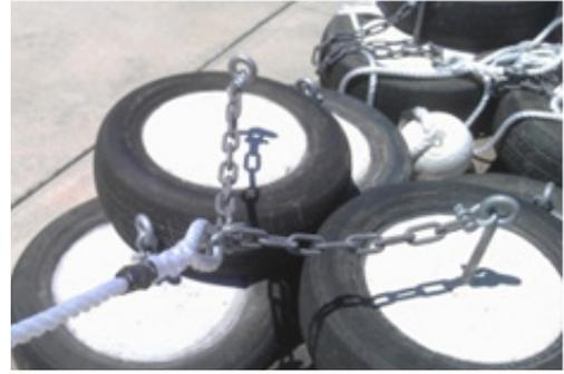
The holding strength required from the anchors will depend upon the operating conditions. In the case where large anchoring forces are required and it is impractical to deposit large and heavy anchors, multiple smaller anchors can be used to generate a similar anchoring weight. Ideally, anchors are placed (embedded where possible) in new ponds prior to filling.
